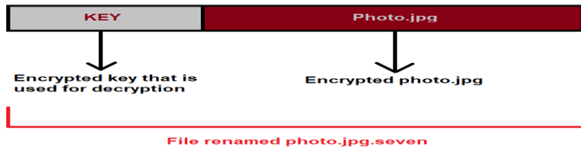
Fig. 5. Overview of the structure of encrypted files.[26]
